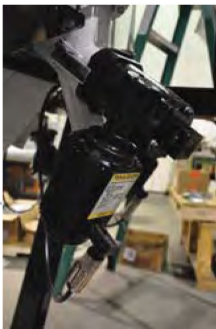
Brushless Gearmotor installed on an X Series Continuous
